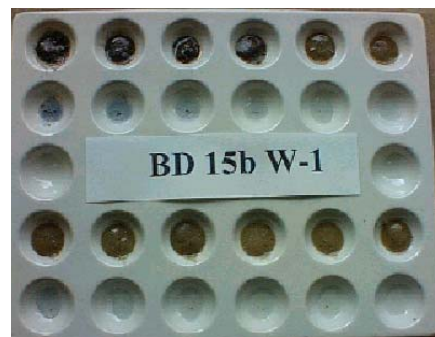
Example of the colorimetric procedure used in the P quick test
