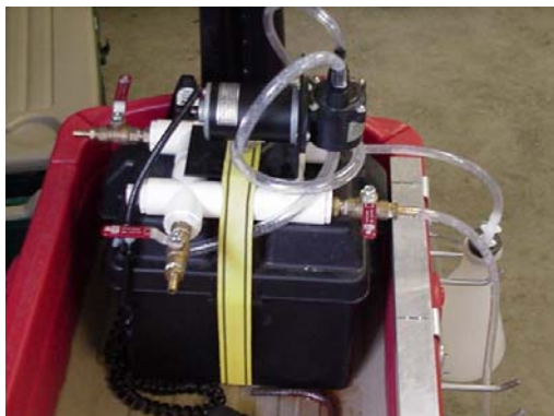
Figure 1. Pump used to collect leachate from turf plots
