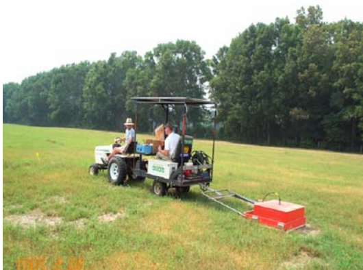
The GPR at work at one of the dairy sprayfields in the study
