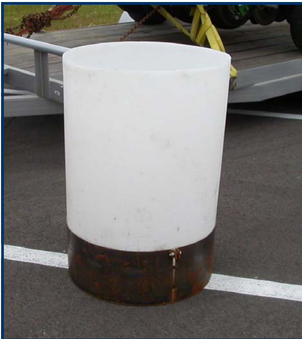
Lysimeter to be used for DEP turfgrass nutrient leaching research. Lysimeters are buried to a depth of 3'. Sampling will be conducted twice a week.
