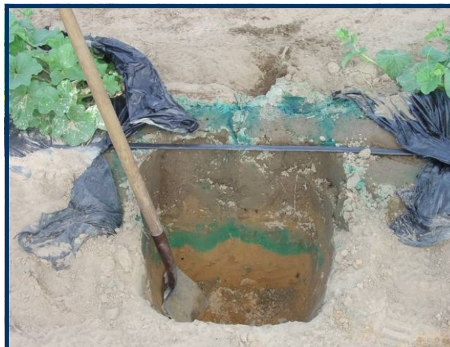
Visualization of water movement in a muskmelon field using soluble dye on May 14, 2004 on an Orangeburg fine sandy loam. Note the dye accumulated above the impermeable layer.
