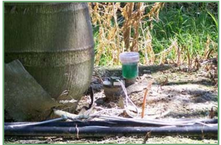
Figure 1: Tensiometer installed in field nursery
